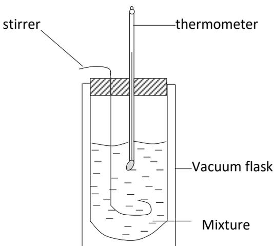
NB. A vacuum flask is used to minimize heat losses
